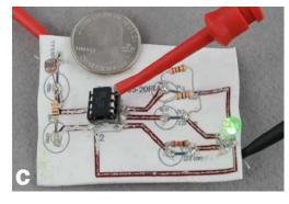
Figure 5: A ShrinkyCircuit designed using Eagle PCB software. a) Electronic components loaded on a circuit printed on polymer sheet with inkjet printer. The electrical connections are traced with a connective pen. c) IC holder is inserted into the shrunk circuit after the polymer substrate is heated. d) The ShrinkyCircuit under operation.
