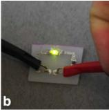
Figure 4: ShrinkyCircuit with surface-mount components. a) Circuit board after the components are loaded with conductive epoxy. b) The ShrinkyCircuit under operation.
