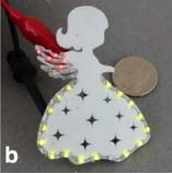
Figure 6: ShrinkyCircuit cut with a low-cost vinyl cutter. a) Polymer substrate prior to shrinking. b) ShrinkyCircuit under operation.
